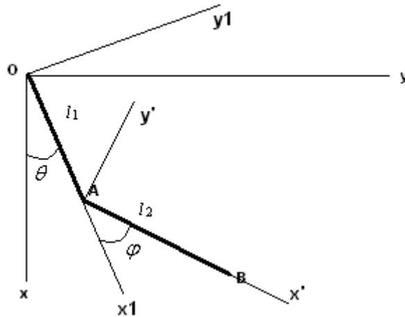
$R_0 = Oxyz$  repère fixe,  $R_1 = Ox_1y_1z_1$  repère mobile  $\vec{\omega}_{R_1/R_0} = \dot{\theta} \vec{k}$
