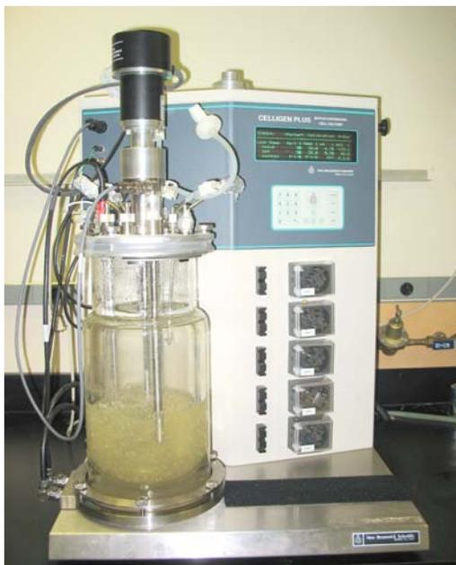
Fig. 1. New Brunswick Celligen-Plus mechanically agitated bioreactor with a 2.5 L working volume.
