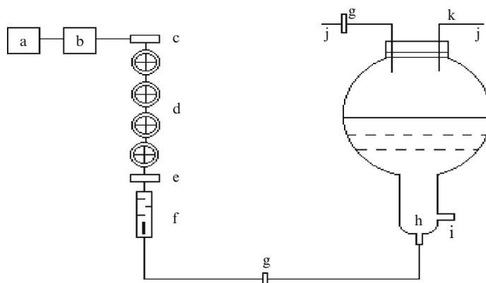
Fig. 1. Schematic diagram of an air lift bioreactor. (a) air compressor, (b) air reservoir, (c) air cooling device, (d) air filter system, (e) air dryer, (f) air flow meter, (g) membrane filter, (h) glass sparger, (i) medium sampling port, (j) vent, (k) pre filter.
