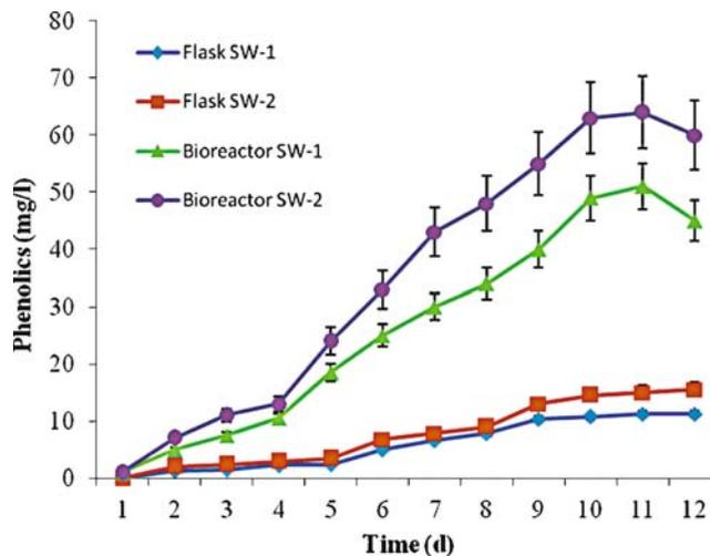
Fig. 5. Phenol production in shake flask cultures vs bioreactor grown cell suspensions of sandalwood. Average of three replications; the maximum standard deviation was less than 8%.
