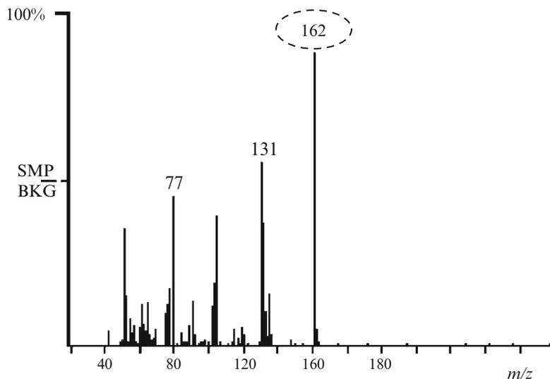
Fig. 2. Mass spectrum (EI mode) of the safrole peak, from the GC-MS analysis of an organosolvent extract of *Ocotea odorifera* cell suspension cultures, showing the base peak being the molecular ion (162  $m/z$ ), consistent with the mass spectrum of authentic safrole.
