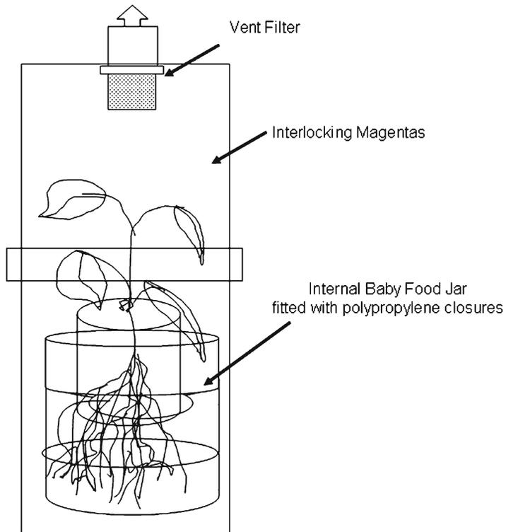
Fig. 1. The plantlet culture chamber. Plantlet is positioned in baby food jar holes drilled in the polypropylene closures within two interlocking Magenta containers. Root portion of plantlet is completely submerged in media and separated by a polypropylene barrier from the shoot portion which is erect in the atmosphere. Atmospheric alteration is achieved by administrations of air treatments through the vent filter.
