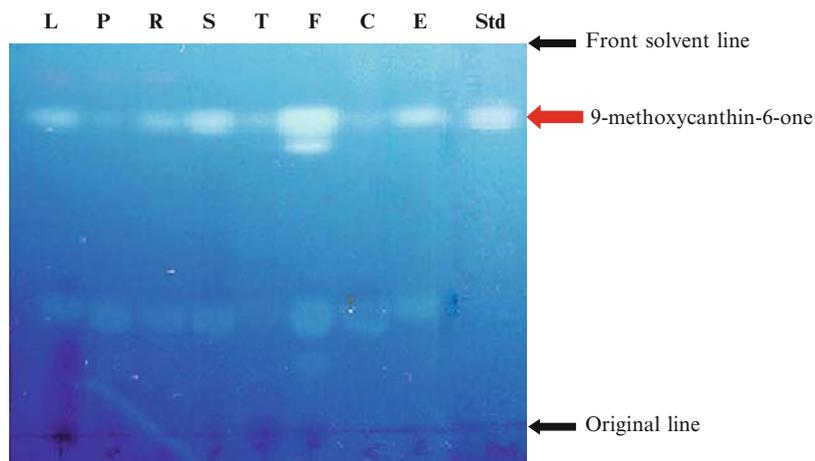
Fig. 3. TLC of 9-methoxycanthin-6-one on aluminium sheets coated with Silica gel 60 F<sub>254</sub> and developed using chloroform and methanol solvent (Callus cultures). The quantity spotted to the active TLC plate was 1.5  $\mu\text{L}$  each. L, Leaf; P, Petiole; R, Rachis; S, Stem; T, Tap root; F, Fibrous root; C, Cotyledon; E, Embryo; Std, Standard 9-methoxycanthin-6-one. The  $R_f$  value of 9-methoxycanthin-6-one was 0.83.
