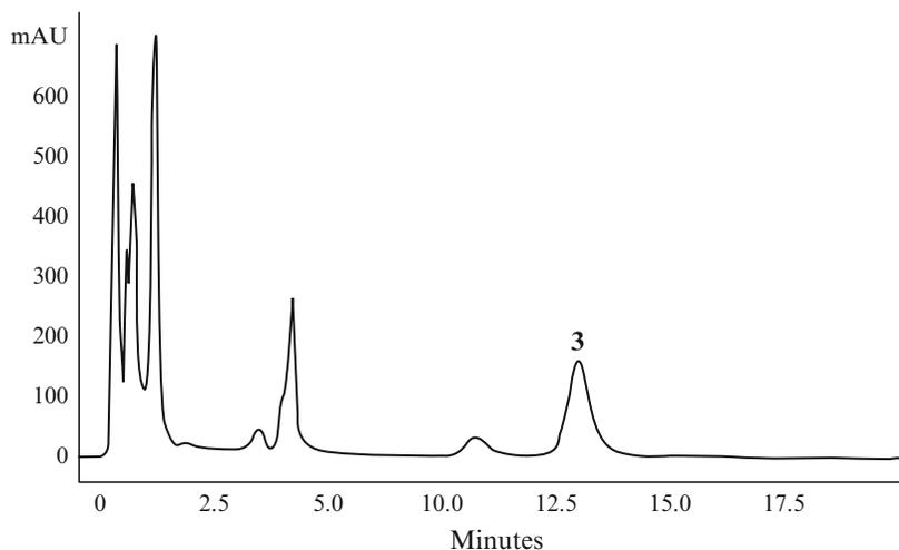
Fig. 4. HPLC profile showing 9-methoxycanthin-6-one peak (peak no. 3).
