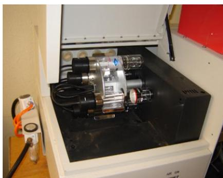
**Fig. 3 :** Source de radiation
