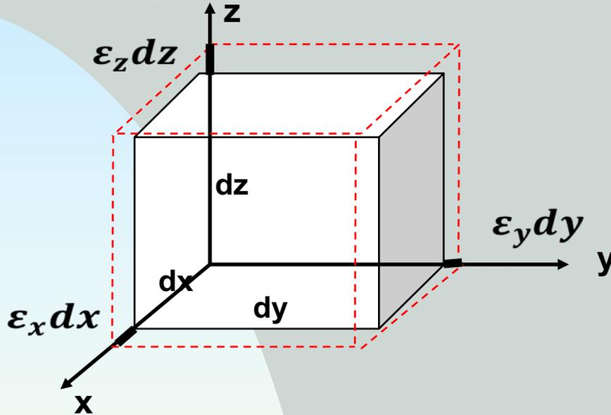
$$[\varepsilon] = \begin{bmatrix} \varepsilon_x & \frac{1}{2}\gamma_{xy} & \frac{1}{2}\gamma_{xz} \\ \frac{1}{2}\gamma_{xy} & \varepsilon_y & \frac{1}{2}\gamma_{yz} \\ \frac{1}{2}\gamma_{xz} & \frac{1}{2}\gamma_{yz} & \varepsilon_z \end{bmatrix}$$
