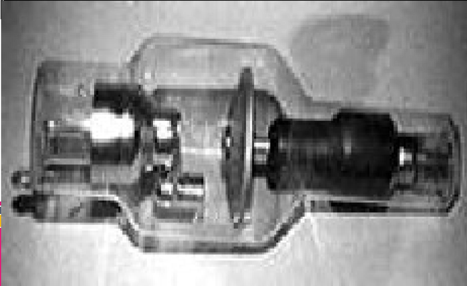
Tube a Anode tournante
