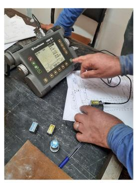
**Ultrasonic Testing (UT) Equipment**
