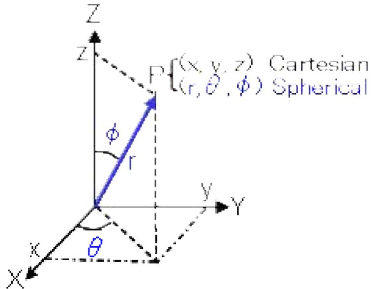
Spherical coordinate robot has one prismatic joint and two revolute joints to positioning parts/objects. These are extensively used in industries in FMS.
