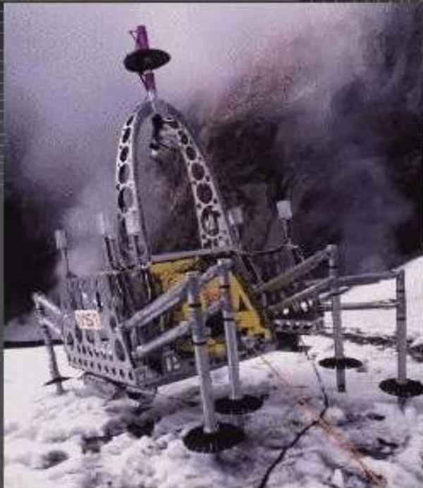
Dante 2, a NASA robot designed to explore volcanoes via remote control.
