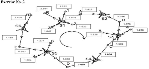
A surveyor conducted a direct leveling survey by traversing through the points: R, A, B, C, D, E, and R'. The points 1, 2, 3, 4, 5, 6, and 7 radiating from stations S1, S3, and S5 as shown in the figure. Calculate the elevations of points: R, 1, 2, 3, A, B, 4, 5, C, D, 6, 7, E, and R'.
