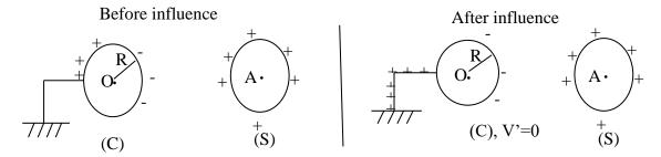
After the influence, positive charges flow to ground and the conductor (C) will have a negative charge and zero potential.  $V_C$ '=0
