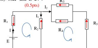
$$\frac{1}{R_{34}} = \frac{1}{R_3} + \frac{1}{R_4} = \frac{1}{6} + \frac{1}{12} = \frac{3}{12} \Rightarrow R_{34} = 4\Omega \text{ (0.5pts)}$$
