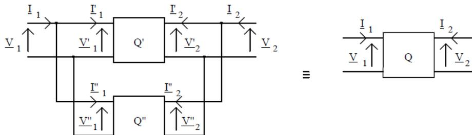
$$Q' \begin{cases} I'_1 = Y'_{11}V'_1 + Y'_{12}V'_2 \\ I'_2 = Y'_{21}V'_1 + Y'_{22}V'_2 \end{cases} \quad Q'' \begin{cases} I''_1 = Y''_{11}V''_1 + Y''_{12}V''_2 \\ I''_2 = Y''_{21}V''_1 + Y''_{22}V''_2 \end{cases} \quad \begin{cases} V_1 = V'_1 = V''_1 \\ V_2 = V'_2 = V''_2 \end{cases} \quad \begin{cases} I_1 = I'_1 + I''_1 \\ I_2 = I'_2 + I''_2 \end{cases}$$
