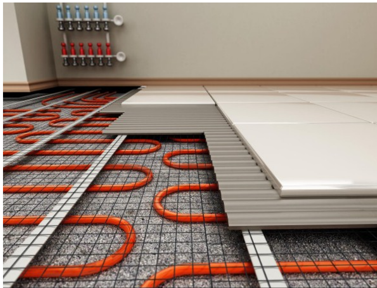
Figure 34. Le chauffage au sol (source : https://www.chauffageavenue.com )
