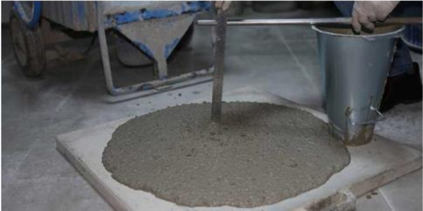
Self-compacting concrete fluidized with a superplasticizer
