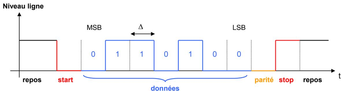
$$\text{Horloge} = F = \frac{1}{\Delta} \text{ Hz}$$
