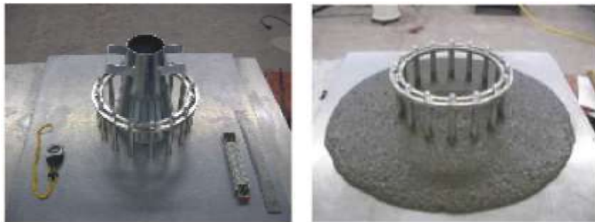
Figure 1.10 : (a) Japanese Ring (J-Ring) and Abrams Cone , (b) J-Ring (Holcim, 2004)
