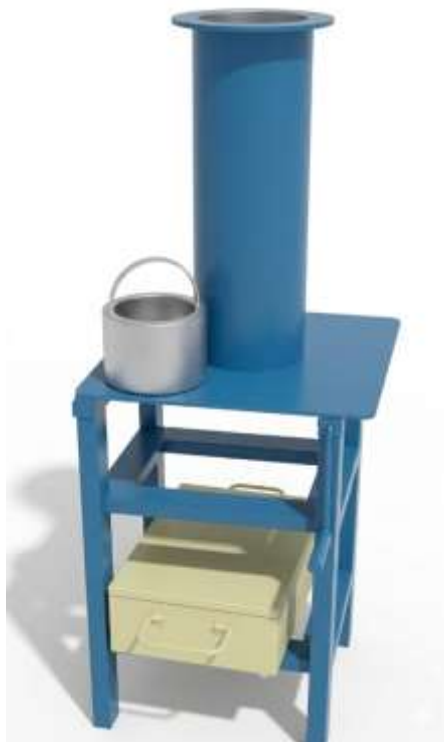
Figure 2.7 : Test bench for compactness measurement
