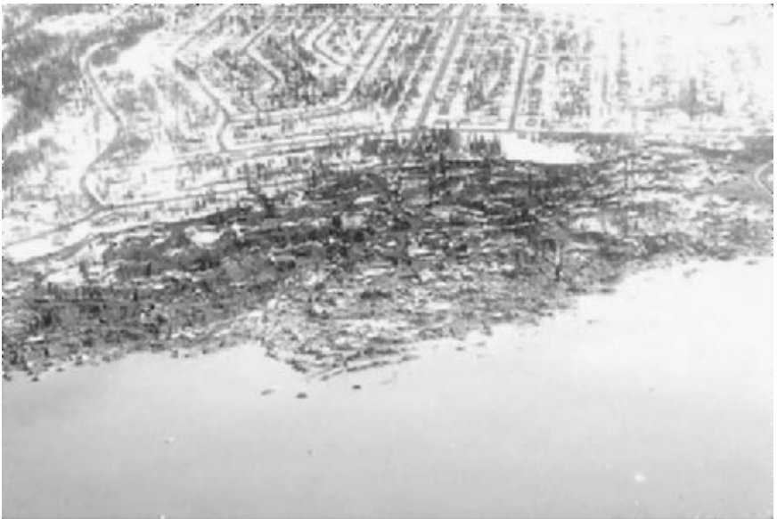
FIGURE 3.45 Aerial view of the Turnagain Heights landslide caused by the Prince William Sound earthquake in Alaska on March 27, 1964. (Photograph from the Steinbrugge Collection, EERC, University of California, Berkeley.)
