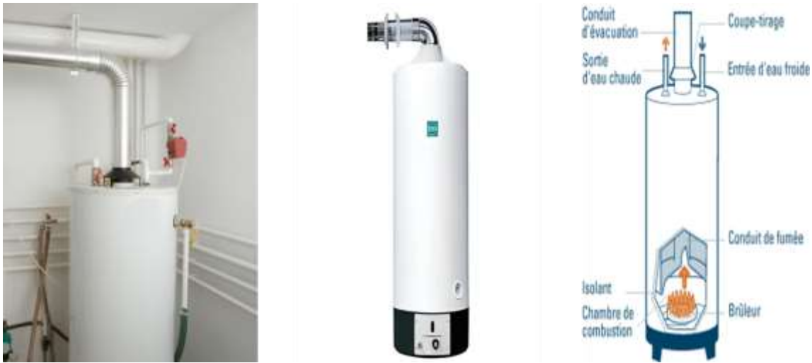
Figure III.4 : Chauffe-eau gaz à accumulation
