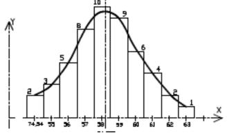
The resulting distribution curve of these measurements always has the same shape and is called a Gaussian curve.
