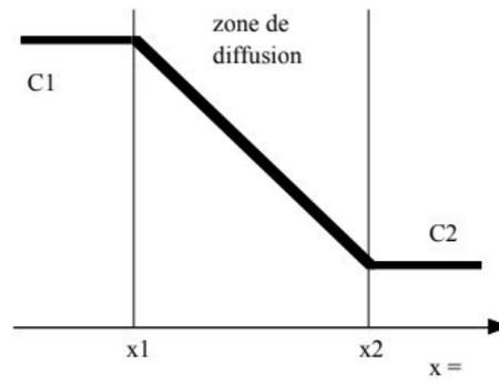
$$\Phi = D S \frac{C_2 - C_1}{x_2 - x_1}$$
